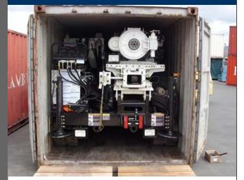
Sonic Drill Corporation, a world leader in sonic drilling technology, recently released a sonic drill rig that is able to fit within a 20' shipping container.
